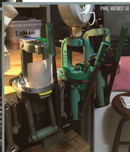
left: A dedicated Redding powder measure, set up for 5.56 reloading.
