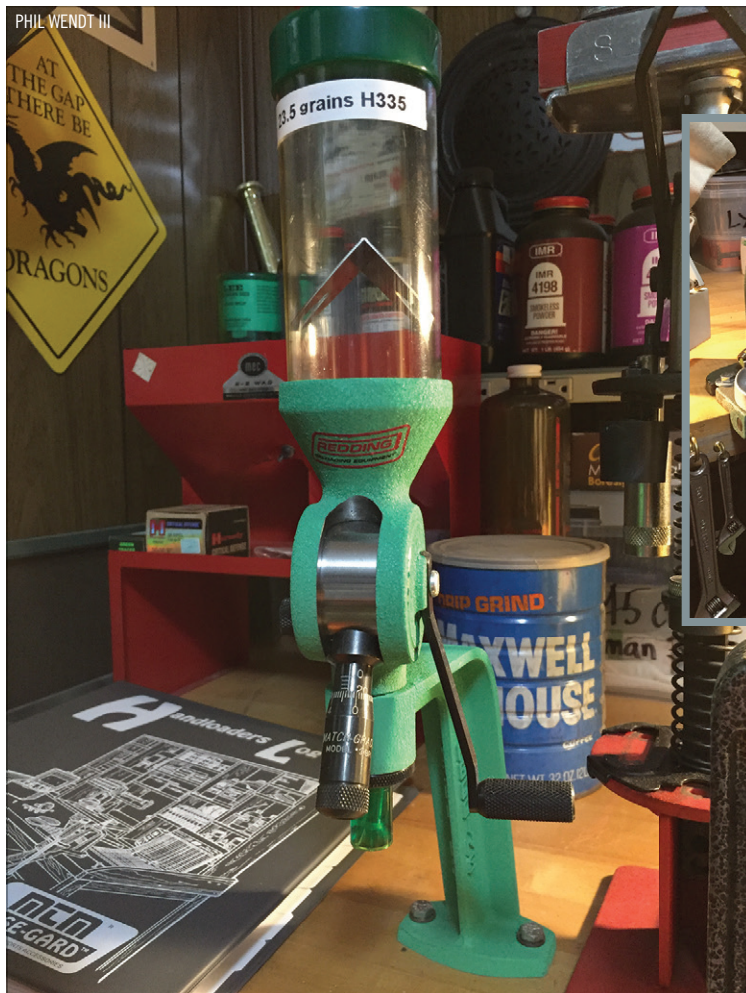
left: A dedicated Redding powder measure, set up for 5.56 reloading.
