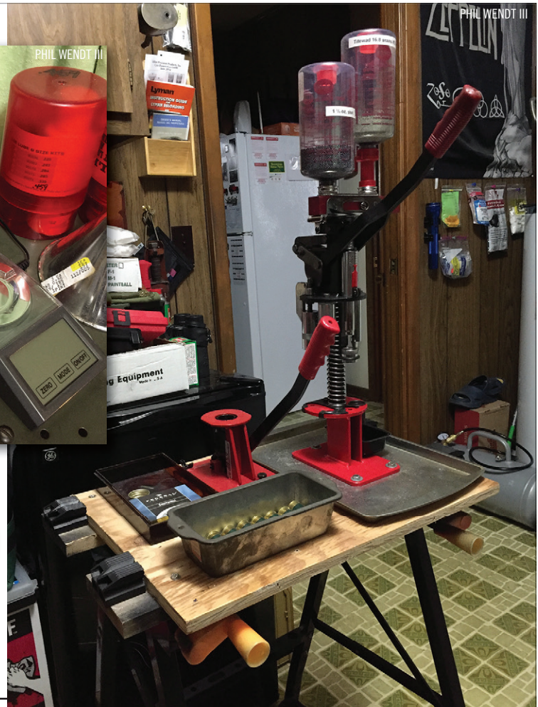
12 gauge shotshell reloading MEC 600 jr set up to reload 1 1/8 oz. loads To the left of the press is a MEC 12 ga. super sizer, a tool that swages the base down fully to ensure positive feeding and extraction in tight shotgun chambers.
